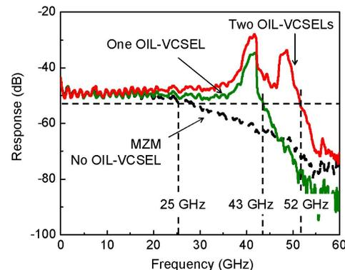
Fig. 4 A resonant frequency response of externally modulated COIL. Bandwidth of  $\sim 52$  GHz is achieved.
