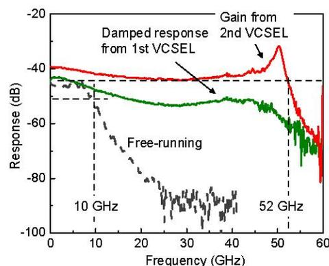
Fig. 2 Frequency response of COIL when the VCSEL is modulated. The first stage is red-detuned to result in a damped response. 3-dB bandwidth of 52 GHz is obtained.
