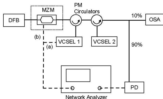
Fig. 1 Experimental Setup (a) direct modulation on the slave laser (b) external modulation on the master laser (MZM: Mach-Zehnder modulator, PM: Polarization maintaining, PD: Photodetector, OSA: optical spectrum analyzer)
