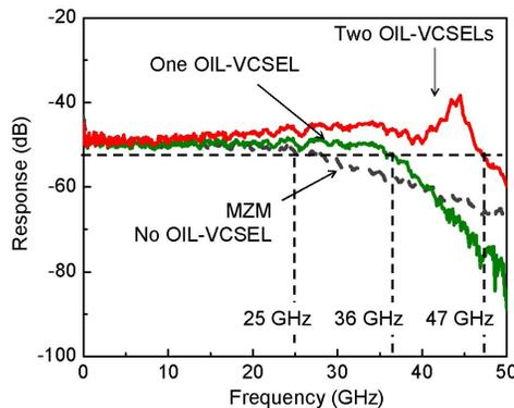
Fig. 3 A damped frequency response of externally modulated COIL. Bandwidth of  $\sim 47$  GHz is achieved.
